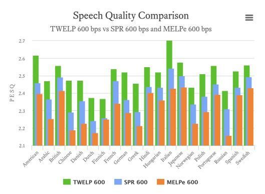
A diagram demonstrates superiority of the SPR 600 bps over MELPe 600 bps in speech quality in clear channel. TWELP 600 bps vocoder provides the best speech quality, but consumes much more (~3 times more) computing resources and memory in comparison with SPR 600 bps vocoder. Exact numbers of the speech quality are presented in the table below.
