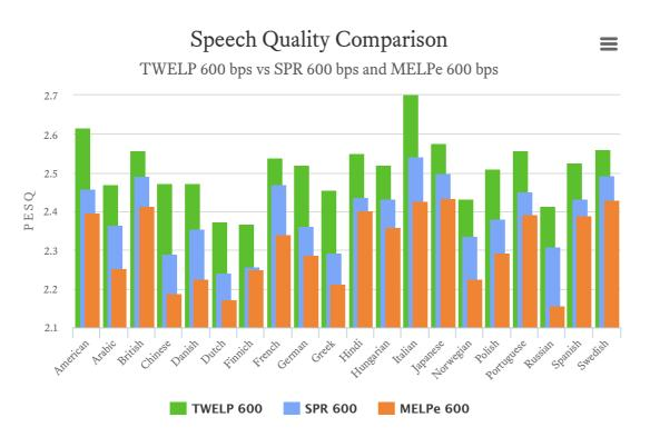
A diagram demonstrates superiority of the SPR 600 bps over MELPe 600 bps in speech quality in clear channel. TWELP 600 bps vocoder provides the best speech quality, but consumes much more (~3 times more) computing resources and memory in comparison with SPR 600 bps vocoder. Exact numbers of the speech quality are presented in the table below.
