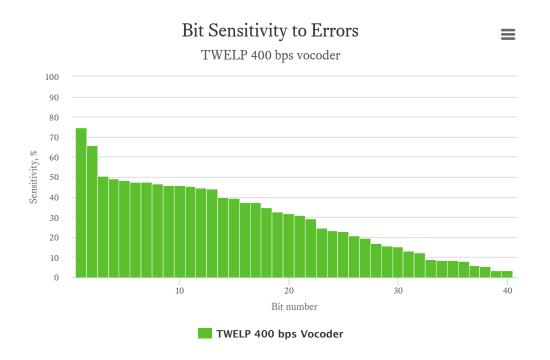
We strongly recommend using FEC (Forward Error Correction) with unequal protection of the bits in strong accordance with their sensitivity to errors and utilizing 'Soft Decisions' decoding. This will provide the highest robustness of the vocoder against errors in the channel.
