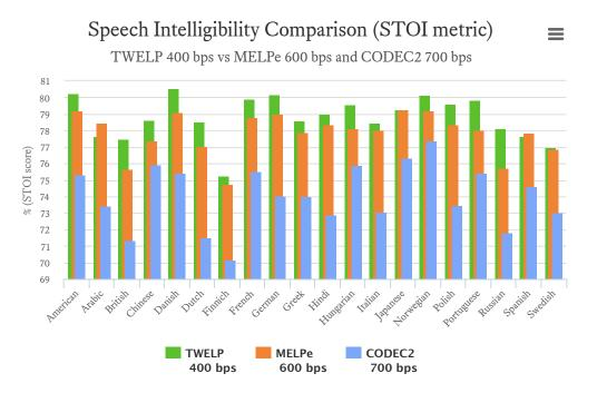
The diagram illustrates a difference in speech intelligibility between the TWELP 400 and MELPe 600 vocoders in the STOI metric. We've also included numbers for the free CODEC2 700 bps vocoder for comparison. Exact values are provided in the table below:
