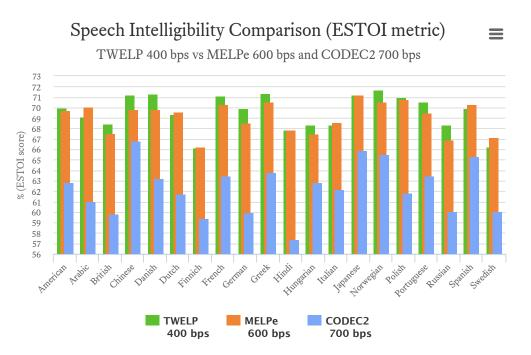
The diagram shows a difference in speech intelligibility between the TWELP 400 and MELPe 600 vocoders in the ESTOI metric. We've also included numbers for the free CODEC2 700 bps vocoder for comparison. Exact numbers are shown in the table below.
