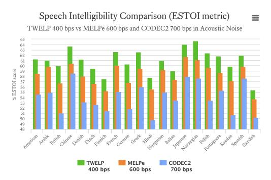
The diagram demonstrates a difference in speech intelligibility for noisy speech (SNR = 10 dB) between the TWELP 400 and MELPe 600 vocoders, based on the ESTOI metric. We've also included numbers for the free CODEC2 700 bps vocoder for comparison. Exact numbers are shown in the table below.
