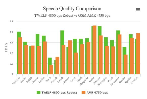
A diagram demonstrates superiority TWELP 4800 Robust vocoder over GSM AMR 4750 vocoder in speech quality in clear channel. Exact numbers are shown in the table below.
